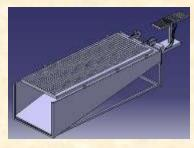
A demonstration of design and fabrication of solar based sand sieving system is done. This system puts forward a fully automated sand filtering and separator that automatically filters the sand poured on it. For this a motorized shaft is mounted horizontally on the mounts. The shaft is connected to a filter frame with a mesh below and enclosed frame on sides which operates the motor when switched on.
