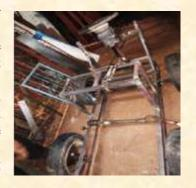
Coordinated four wheel steering help in parking and low-speed manoeuvres efficiently due to the rear wheels turning contradictory to front wheels and this helps in achieving a smaller radius of turning. At higher speeds, all the four wheels steer in the same direction in order to achieve more stability and less body lean during fast lane changing.
