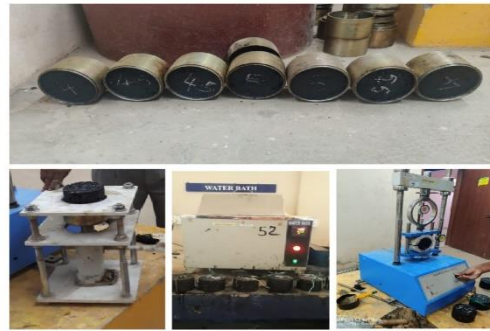
fig2.Marshall stability testing apparatus.
