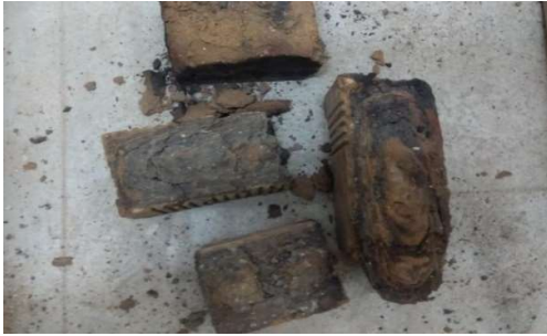
Fig (ix) Bricks made with black cotton soil
