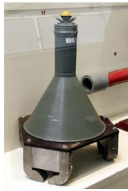
Fig 15 : The german made Hafthohlladung is a anti tank mine made up of magnetic components
