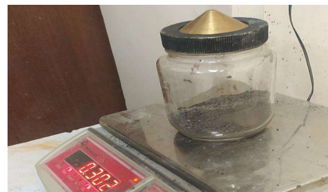
Fig (v) Soil in pycnometer
