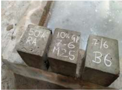
Figure 6. Cubes casted at laboratory
