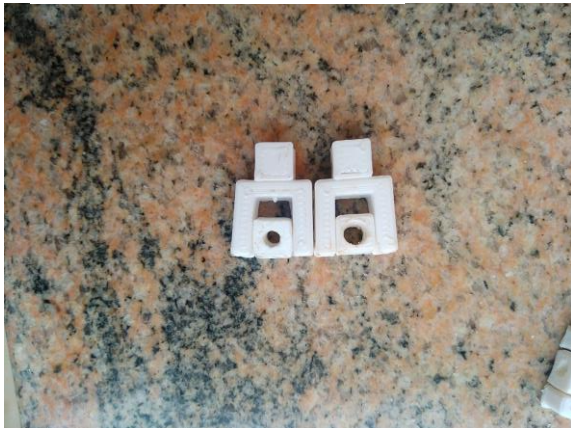
Figure 3: Universal Joint, 3D Printed
