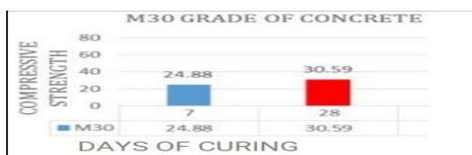
GRAPH SHOWING THE COMPRESSIVE STRENGTH OF M30 GRADE OF CONCRETE MIXED WITH SCBA
