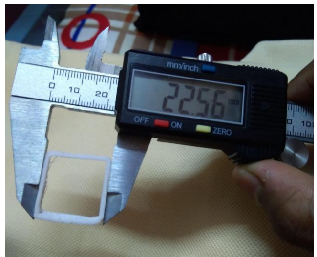
Figure 9: A test part showing the dimensional accuracy of the machine
