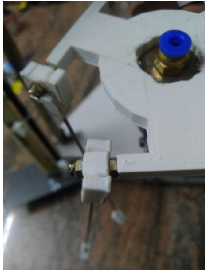
Figure 8: End Effector, designed in-house
