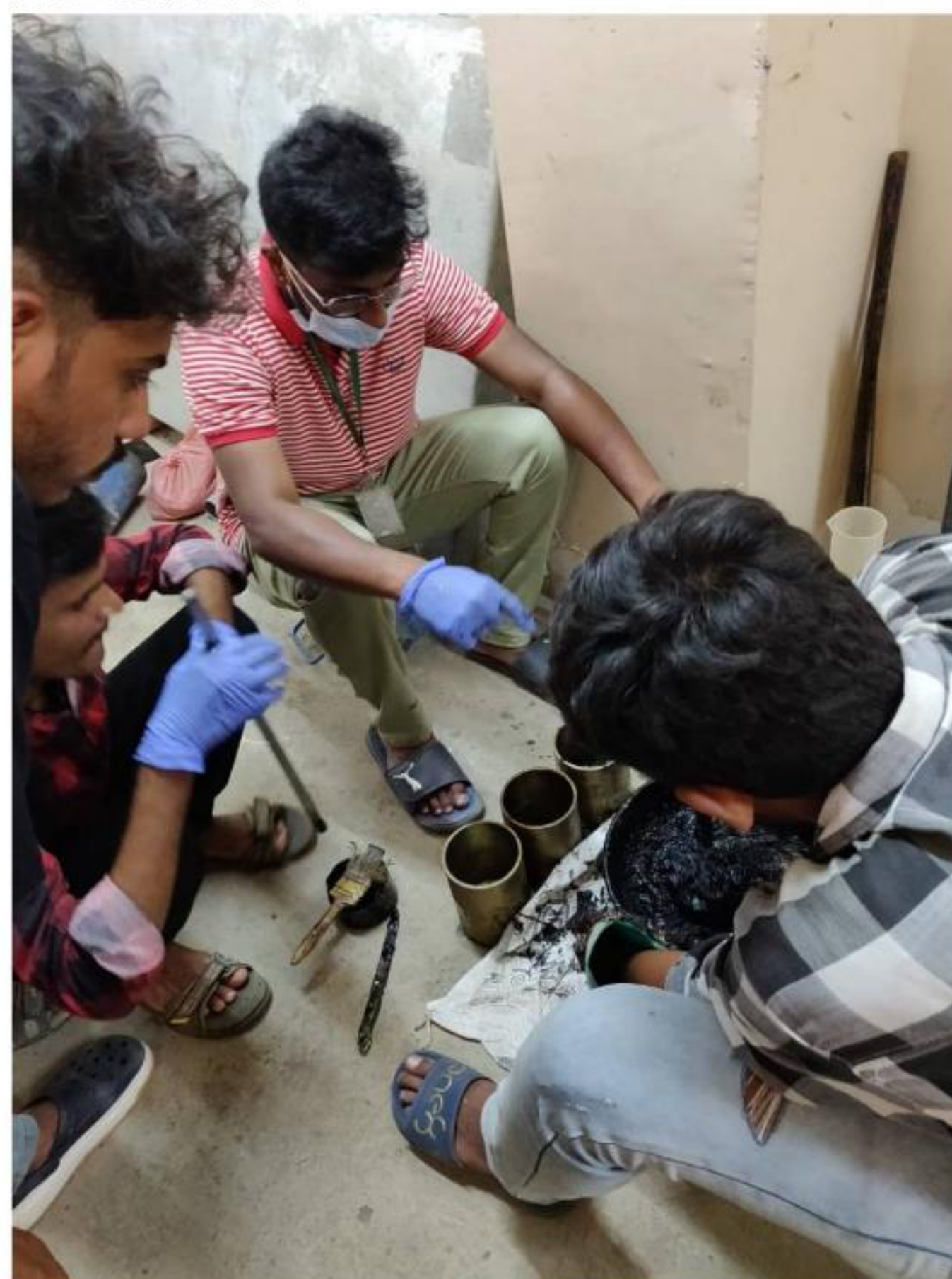
FIG.2 CASTING THE SPECIMEN INTO THE MOULD
