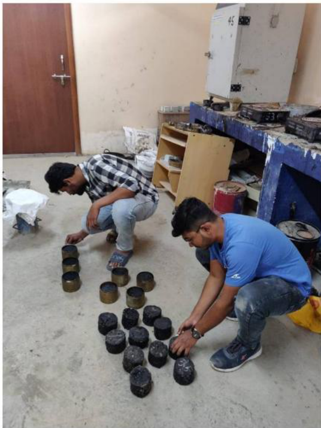
FIG.3 UNMOULDING SPECIMEN AFTER 24 HOURS OF CASTING
